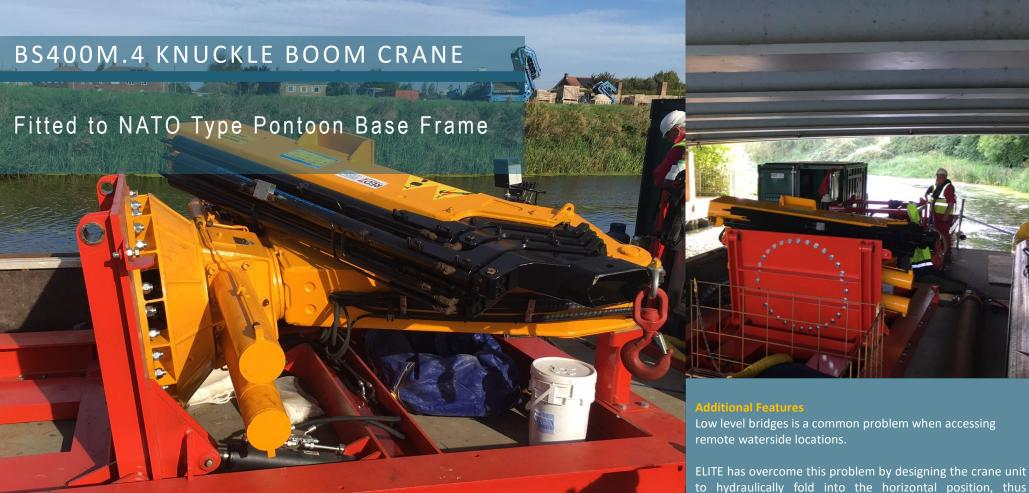
to hydraulically fold into the horizontal position, thus allowing barges to traverse under low level bridges and obstacles with low headroom. The crane can be folded back into the working position within minutes.
